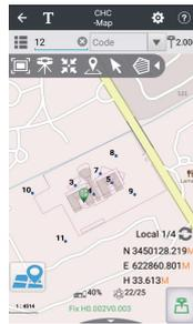
**Convenient** work mode management: Supports presetting of common work modes of base and rover, selecting or switching work modes by one button push. You will not need additional steps to configure your work mode while surveying. The streamline user interface designed to be operated with your fingers.
