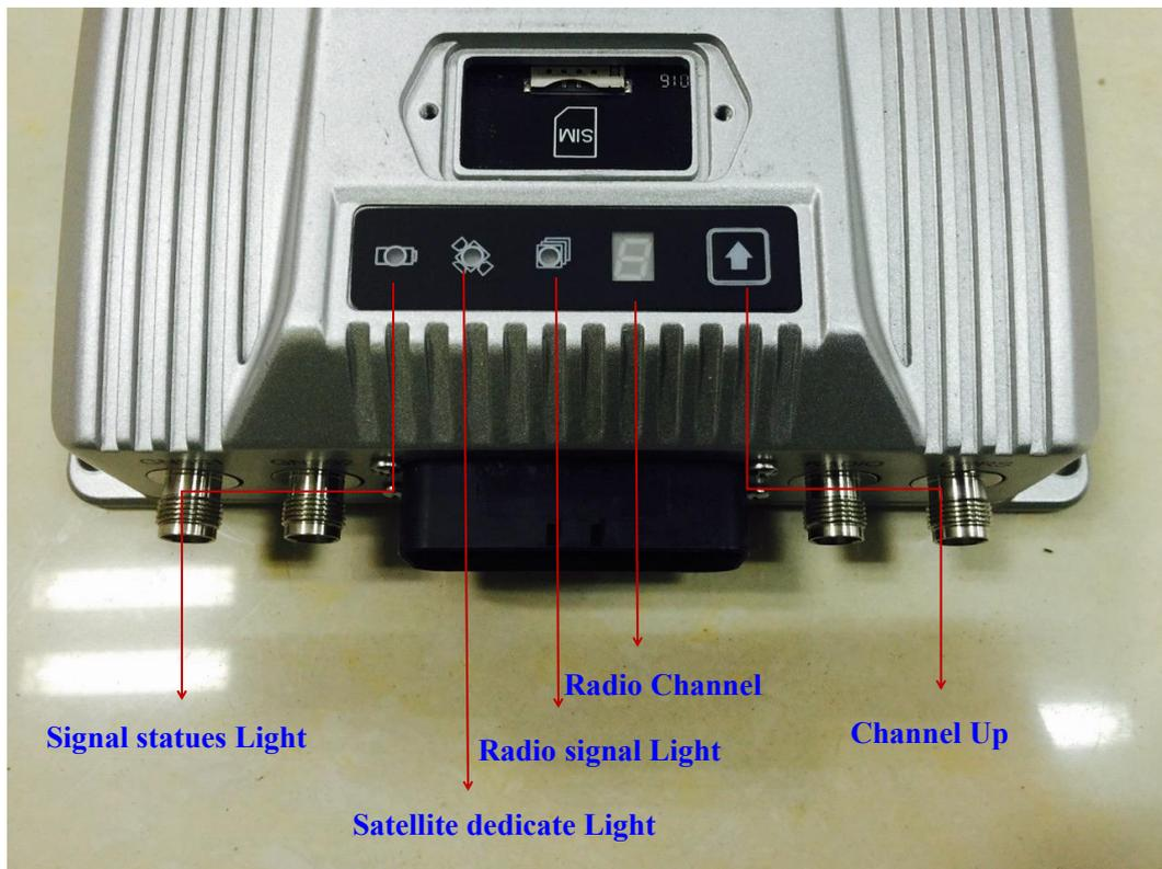
The right button is the FM button, from left to right fourth yellow (the power after the color) light for the radio signal, the yellow lantern flashes several times continuously, then flashes the same number of times every other time, the yellow light flashes several times for several channel base station signal continuously, for example: yellow lamp each paragraph is continuously blinks 5 times, namely
