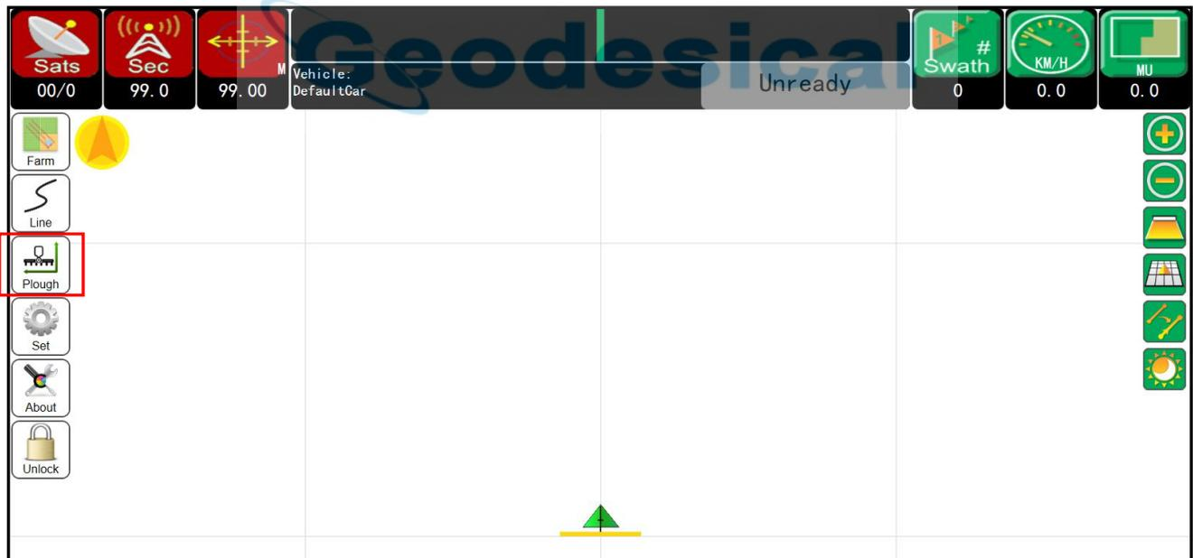
1. In the center offset, enter the sum of the current value and the previous calculation offset, and note the positive and negative numbers in the calculation. (that is, the left side of the farm tools is positive, the right side of the farm tools are negative)
