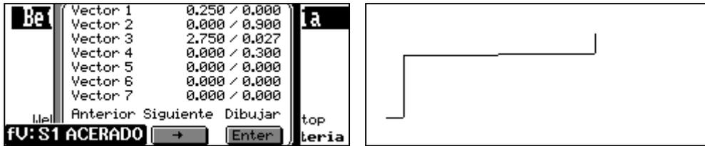
Here is an example of a disassembly with a berm that rises up while changing slope inclination of 1/1 at the outer side to 2/1 on the inner side:
