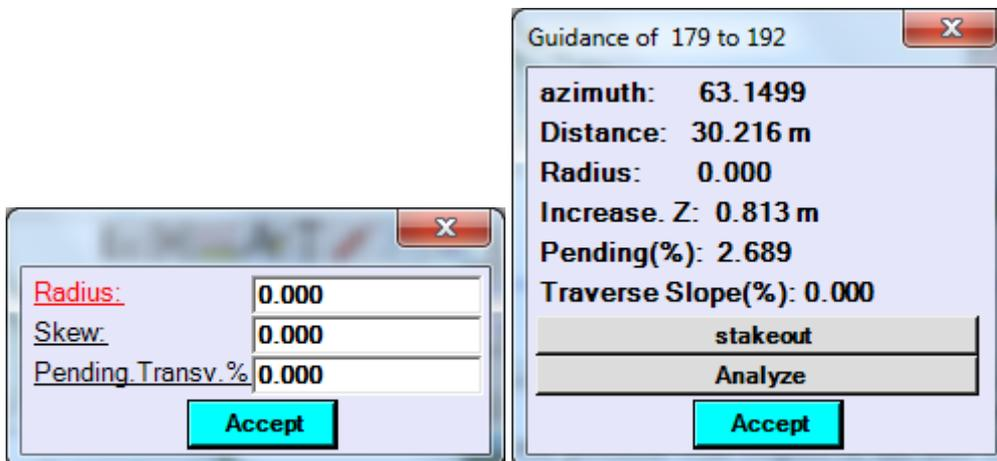
**A.- Stake:** Requests a Pk, distance to the axis, Z increment, transverse, and progressive slope as the Pk increases.
