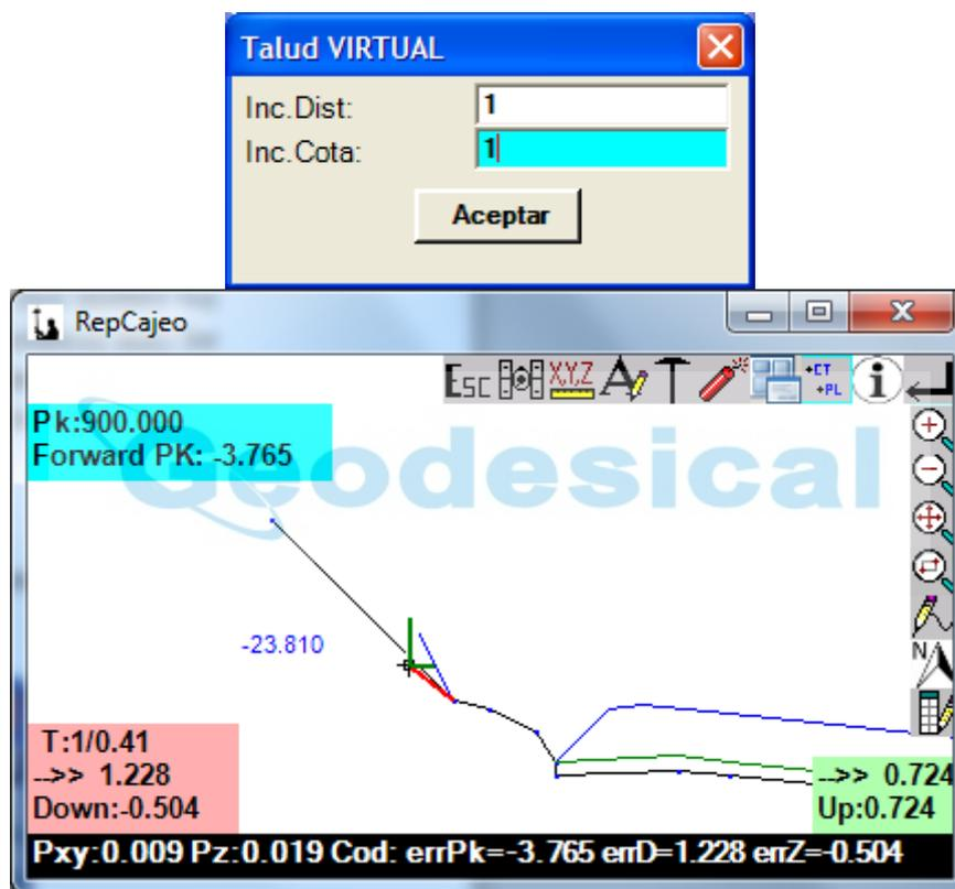
In this example we have defined a vector 1/1 that starts at the ditch and is more sloped than the original (1/0.5), if we move until the data at the bottom right is ZERO we are at the intersection of the Virtual Slope and the ground.
