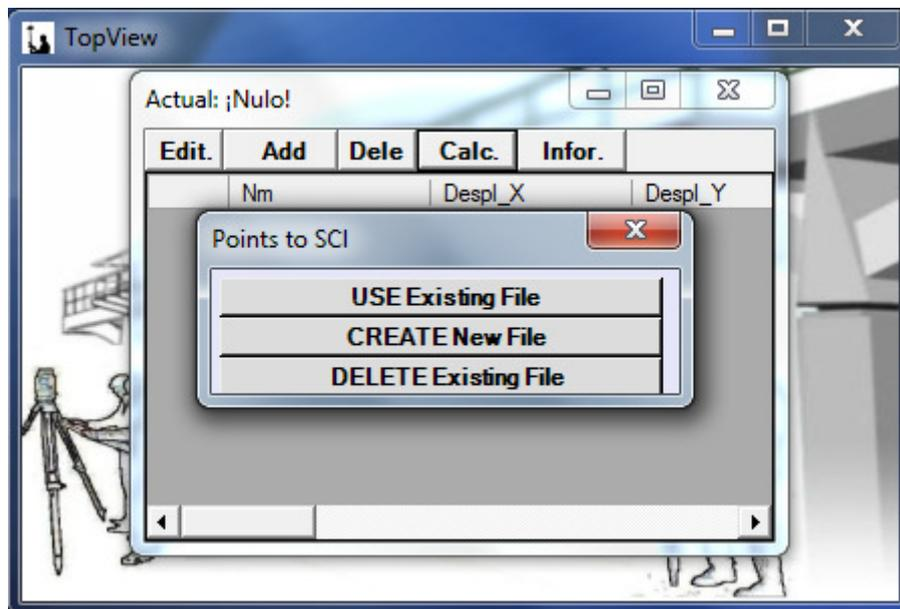
The calculation button creates a file with "Points for SCL" which consists of a register for each Base used for the SCL that has the base name, the Local Cartesian coordinates and the Cartesian coordinates taken by the GPS according to Datum, timezone, and the geoid used for the calculation. This file has the extension \*.dtm and in TopView is shown thus:
