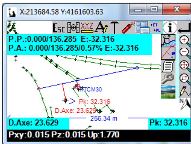
In "Coplanar points" after marking three points that define the plane the program draws the triangle from these three points and shows our position along with calculating the increase to reach the plane, when we're inside or outside it.
