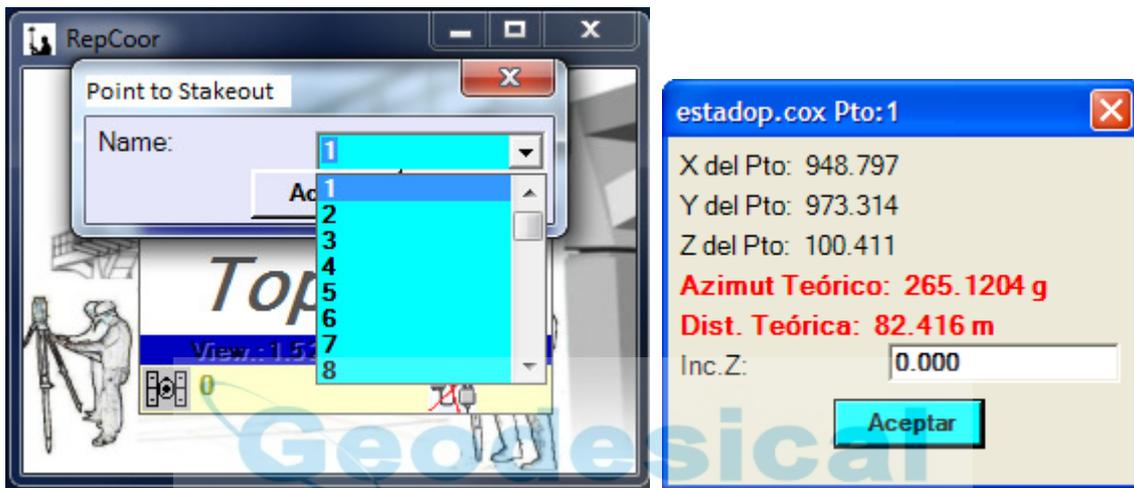
After placing the apparatus with the indicated azimuth and the linear operator, we can check it by pressing Enter. After taking the reading, the program asks for the height of the pole and the code we want to use for the point to save in the backup file.
