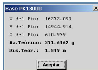
After taking a reading from the device the program informs us of the point with respect to the alignment with the base and the actions to take.
