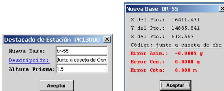
It should be noted that for greater accuracy of the data from the new base, two readings (**direct and reverse**) are taken.
