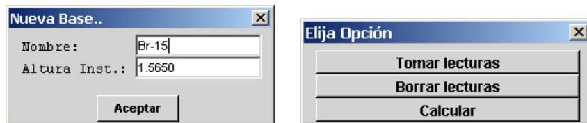
For a greater precision of data from the new base two readings are taken (direct and reverse). The order of the readings is of free choice, with the program being responsible for accurately positioning the new Calculated Base.
