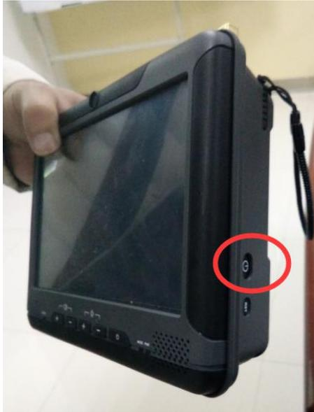
The right switch button on the display is 1 seconds short to open the display
