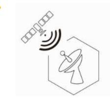
220-channel All Constellation Tracking GPS: L1C/A, L1C, L2C, L2E, L5 GLONASS: L1C/A, L1P, L2C/A, L2P, L3 Galileo: E1, E5A, E5B BDS: B1, B2 SBAS: L1C/A, L5
