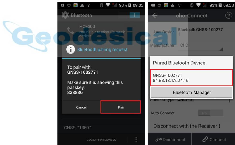
5. Tap the **Connect** button to build the connection.
