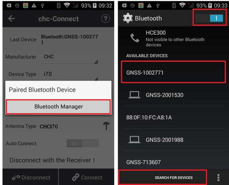
4. Tap **Pair** to connect the bluetooth device → selected the target device in the bluetooth manager list
