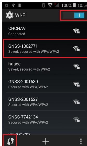
4. Tap **Connect** to link to the hot spot. If the first time connection to this hot spot, user may type in the password.
